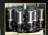
Screen made of a sturdy Aluminium-Magnesium alloy BRAID (AIMg). The braiding process is operated by means of 16 spools braiding machines. The braid plays an important role against low frequency impulsive noises.
